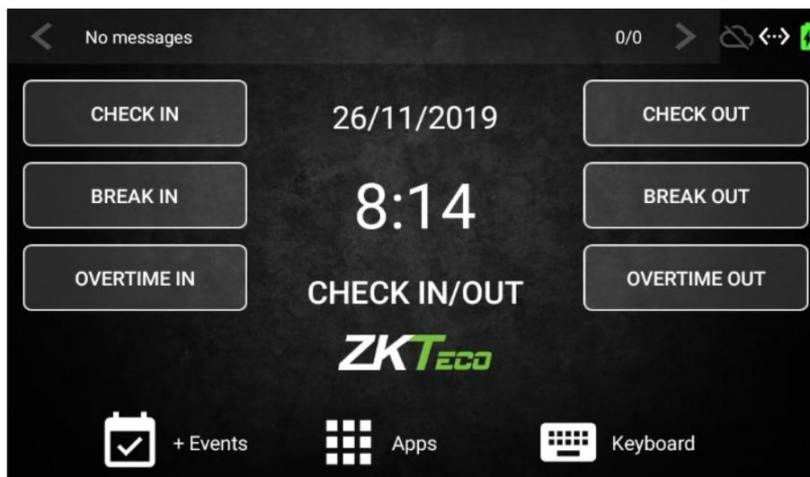
The device has different widgets on the desktop at the factory status: The basic attendance events, which are **Check In, Check Out, Break In, Break Out, Overtime In and Overtime Out**. access to the rest of the functions, which are **+ Events, Keyboard and Apps**, the display of the **Current Date and Time**, the status of the **push communication**, the status of the **network connection** and the **battery status**.
