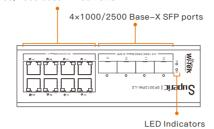
For Hardware V1: Port 1-8 support 802.3af/at PoE output For Hardware V2: Port 1-2 support 802.3af/at/bt PoE output, Port 3-8 support 802.3af/at PoE output
