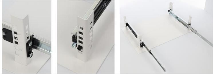
**3.2.** Remove slider and tighten it to ARAD enclosure (M4 screw + washer). The enclosure is to be fixed to the front part of the RACK rails with four M6 screws.
