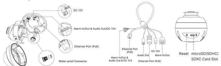
Note: The cable is connected with the interface board by default.
