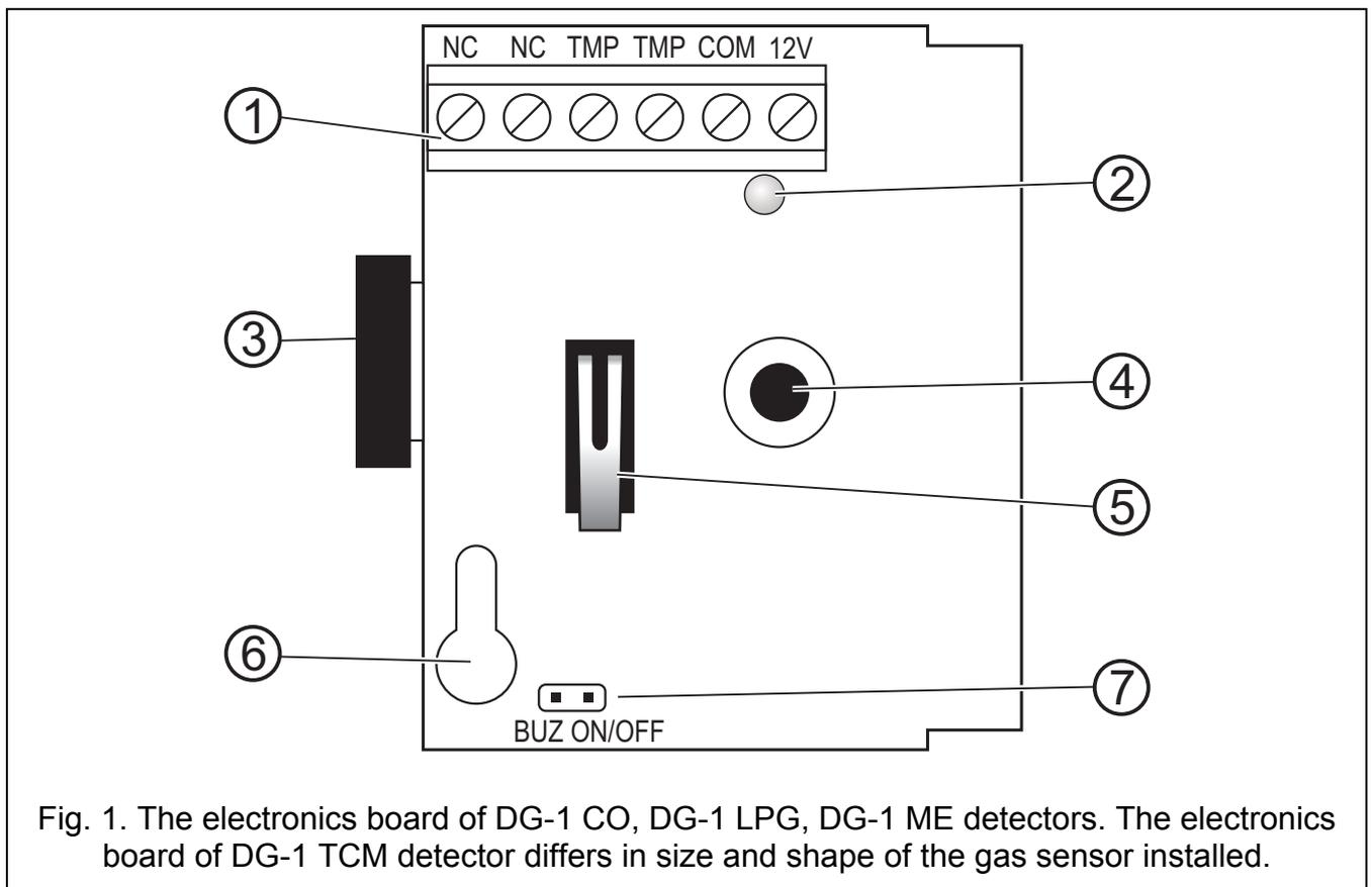
Fig. 1. The electronics board of DG-1 CO, DG-1 LPG, DG-1 ME detectors. The electronics board of DG-1 TCM detector differs in size and shape of the gas sensor installed.
